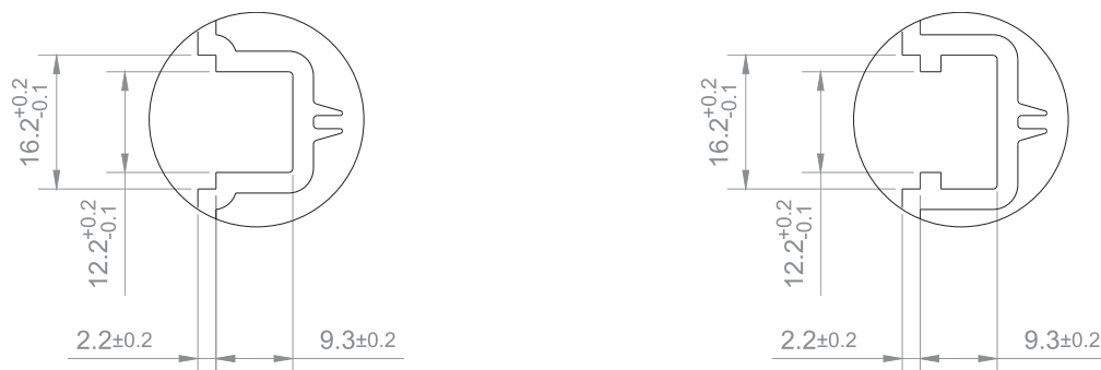
Standard hardware groove dimensions and tolerances
